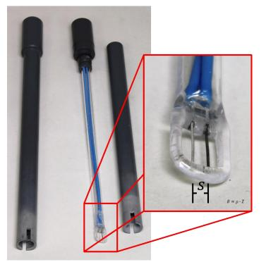
The resistance *R* of the conducting electrolyte solution is dependent on the resistivity  $\rho$  (unit: siemens per meter [S/m]) and the cell constant *Z*.
