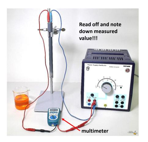
First, the power supply is connected to the conductivity meter.
