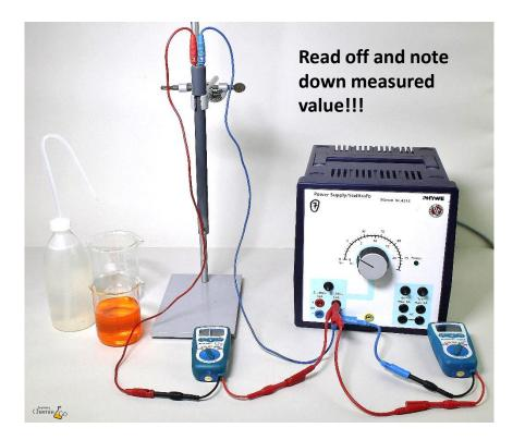
A second multimeter is connected in parallel to measure the voltage. The conductivity meter is immersed vertically into the solution and the measured value is noted down.
